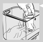
4 Insert the filter into the empty water tank. Press it until it cannot move further down.
