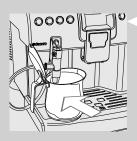
5 At the end of the operation, empty the container and place it under the water dispensing spout.
