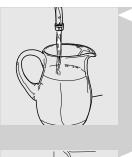
8 Rinse the container thoroughly and fill it with ½ It of fresh water to be used for rinse cycle.
