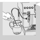
3 Insert the suction tube into the container.
