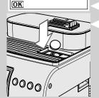
5 Put a "Coffee Oil Remover" tablet in the pre-ground coffee compartment. Press the "" button.
