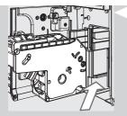
**16** Insert the brew group back into its seat by sliding it along the guides until it locks into place.
