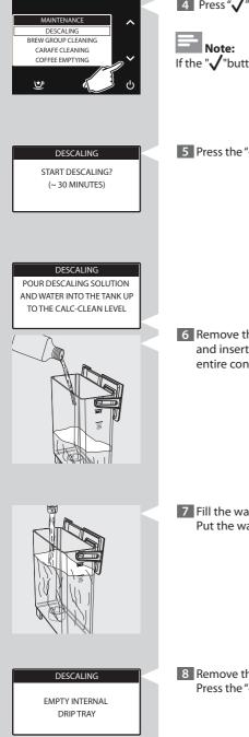
Press " V" to confirm the **"DESCALING"** selection.
