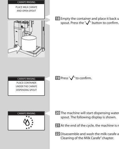
**18** Empty the container and place it back under the coffee dispensing spout. Press the "**√**" button to confirm.
