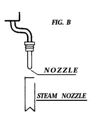
If the machine is not used for extended periods, remove the water in the boiler by pressing the hot water button and opening the tap so that the equivalent of about two cappuccino cups of water flow out of the nozzle. Do this only after the reservoir has been filled with cold water. Never use the pump without water.
